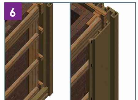
Step 6: If your cladding carries on around a corner, follow Steps 1 through 5. Make sure the External Trim is in the right position, so as to place the Cladding Plank into the right position.
