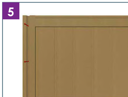
Step 5: Use External Trim, cut to size and secure with screws. If cladding carries on round corner, make sure External Trim lines up with battening. Push in Trim.
