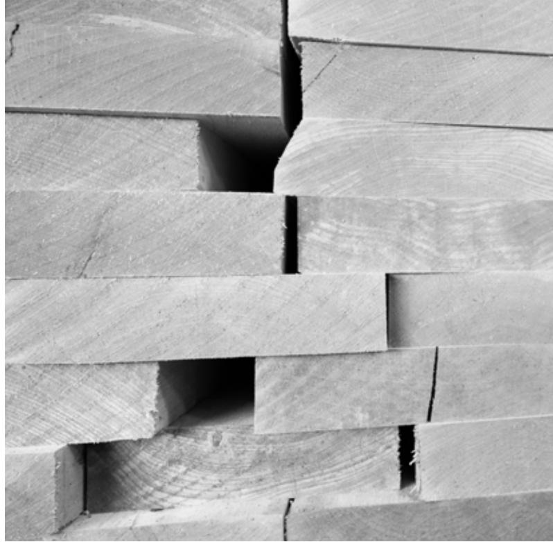
The moisture content of timber can have a profound effect on its performance. Kiln drying is essential for joinery and construction hardwoods and also for clear softwoods that are to be used inside.
