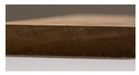
When installing and cutting cross sections, these 'exposed' surfaces do not require additional treatment or sealing. Rhino Wood is modified at a cellular level through to the core, resulting in zero durability weak spots when cutting or fixing on site.
