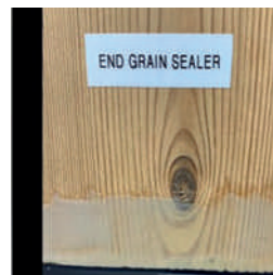
Sealer applied on end grain shows no uptake of moisture in 24hrs
